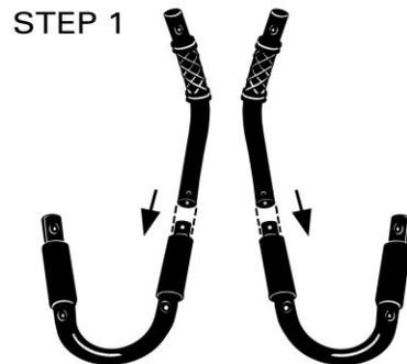
**Step 1:** Insert Left arm into Left Curved Handle. Align drilled holes. Repeat step for right side. Note: Curved Handles are universal.
